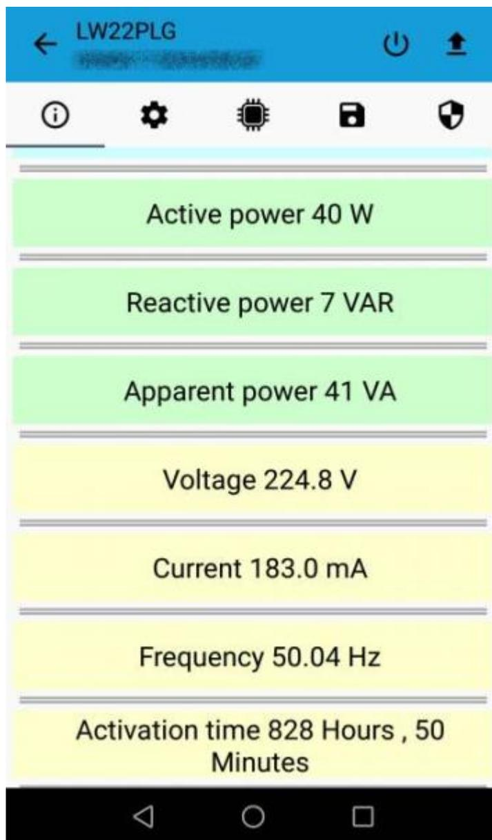
Once provisioned on a LoRaWAN® network, the device sends the measures to the server via uplink.
